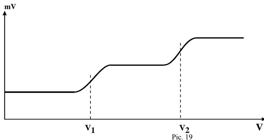
By conductometric titration the values of volume, for which the change of derivative sign appeared, are determined. This are the points of crossing of the straight which approximate the individual segments of the collected series graph (pic. 20).
