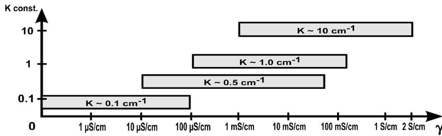
Accurate measurements in the whole range are possible with use of 3 different conductivity cells. The cell with constant  $K \approx 0,1 \text{ cm}^{-1}$  should be used for measurements of ultra pure and redistilled water.
