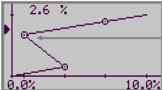
The curve goes backwards because two samples have been exchanged when entering the lab results. Higher Y-value must mean higher X-value. The curve must have a direction upwards and to the right.
