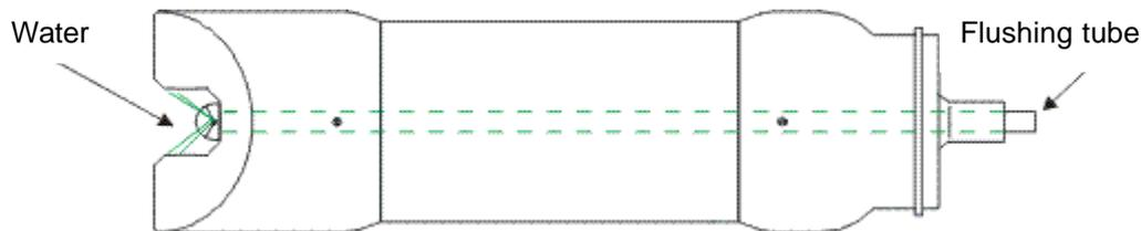
Flushing must be activated in the “Settings” menu in the BB2 control box:
