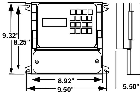
The mounting feet have slots for 1/4" bolts (4 places). The electronics should be mounted with the display at eye level or lower. There are three 1/2" holes in the bottom of the enclosure for conduit fittings. These holes have rubber plugs installed at the factory. If you do not use all three holes for conduit, leave the rubber plugs in the holes to protect the enclosure ratings.
