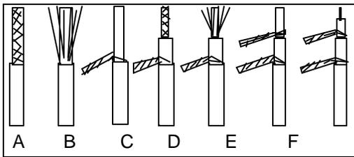
Trim 1 inch of the inner jacket from each of the cables as shown in "D". Again, use care not to cut the inner braid beneath the inner jacket.
