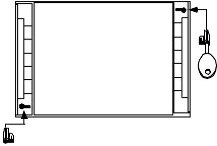
**Note:** The key will have to be left in the hinge handle if the door is to remain unlocked. The only way the key can be removed is if the hinge handle is locked.
