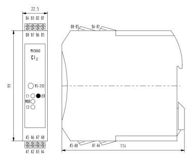
The Transmitter MV 3060 is suitable for direct connection of a electrode/sensor with 2-wire output 4...20 mA especially sensors for disinfectants like chlorine, chlorine dioxide or ozone. Optionally connection of a temperature sensor is possible.
