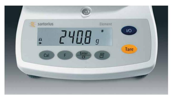
Clear allocation of functions to keys and easy-to-understand symbols enable intuitive operation. The large, white backlit display is exceptionally easy to read. All models include a level indicator and adjustable feet as standard features, for optimal adjustment to the place of installation.
