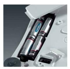
With eight high-capacity 1.5 V batteries in the battery compartment, lengthy measurement series can be performed outside the lab at any time. The hook for below-balance weighing is protected by a plastic cover on the bottom of the balance.
