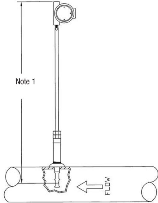
1-1/2" Insertion Meter Assembly with Insertion Tool and Ball Valve
