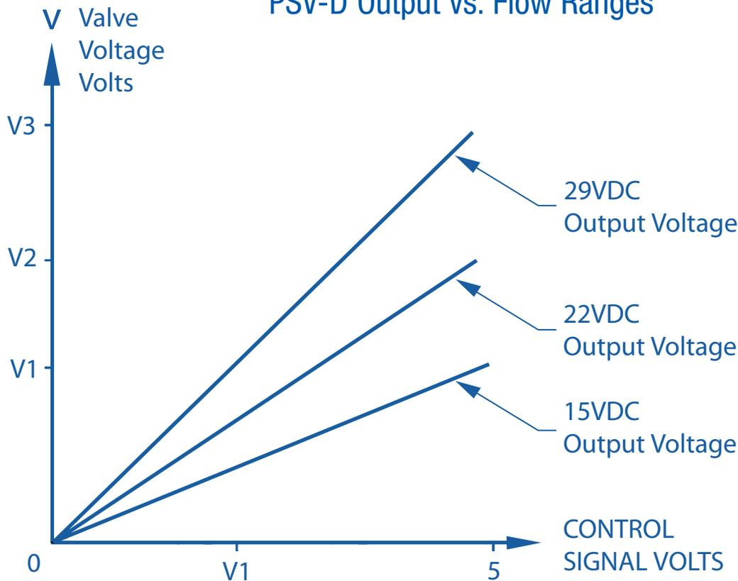
Jumper selectable output power allows a choice of dc voltage range for cooler more efficient operation, as a function of flow rates.
