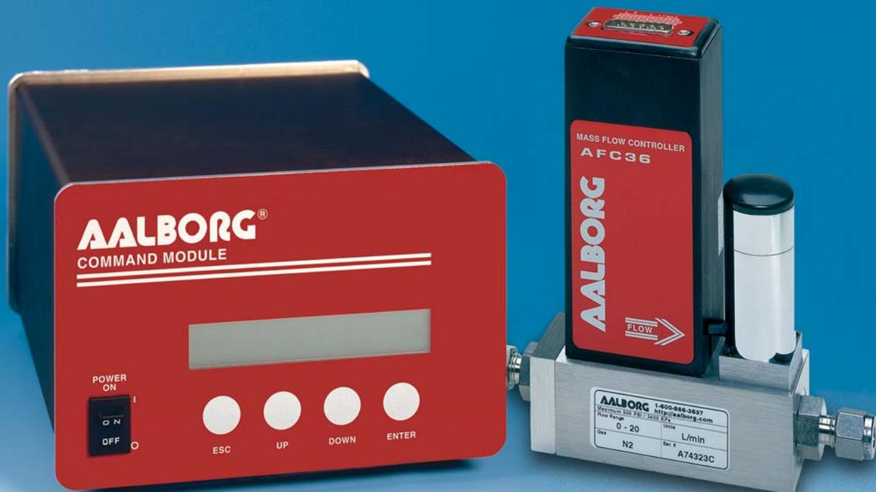
In AFC mass flow controllers the combined gas streams flow through a proportionating electromagnetic valve with an appropriately selected orifice. The closed loop control circuit continuously monitors the mass flow output and maintains it at the set flow rate.
