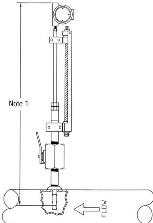
1-1/2" Welded Insertion Meter
