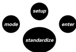
9. To enter a third standard, place the electrode in the third buffer solution, stir, allow to stabilize, and press **standardize**. The results are the same as in steps 7 and 8.
