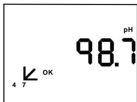
8. **Error** shown with the 'Slope' symbol indicates that your electrode is not working properly. The electrode response must be between 90 and 105%. Measurements that results in 'Slope Error' are not accepted by the meter. Press **enter** to continue.
