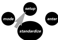
1. Press **setup**; the word *Clear* flashes on the display. *Continue with this step only if you wish to clear all buffers entered.* To clear all existing buffers, press **enter**. The meter clears all buffers and returns to measuring mode.
