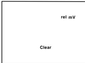
1. To clear the mV offset and return to absolute millivolt mode, press **setup**. The word *Clear* flashes on the display, and the current relative millivolt offset is shown.
