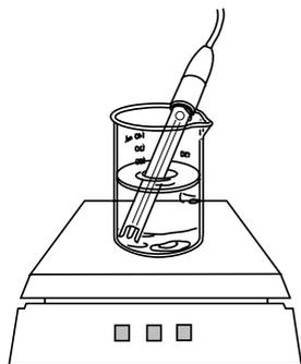
11. Standardize your meter and electrode using at least two buffers with pH values above and below the expected pH of your samples. Stirring with a magnetic stir bar and stirrer provides faster electrode response.
