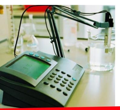
**Calibration data is available for each standardization**. Simply press the Cal Data button for a complete listing of calibration points, time and date of standardization along with electrode efficiencies. Press the graph soft key to see a graph of the calibration curve.
