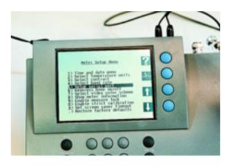
**Great choice for multiple users.** Four features help with uniformity in the use of the meter. Activate the standardization delay and the unit will not complete the standardization process until the programmed time has lapsed. Set the calibration reminder to ensure routine standardization. Use the strict calibration setting to prevent measurements when a calibration is due. Use data alarm to let the meter tell you when data is outside of your range. For further specifications see last page.
