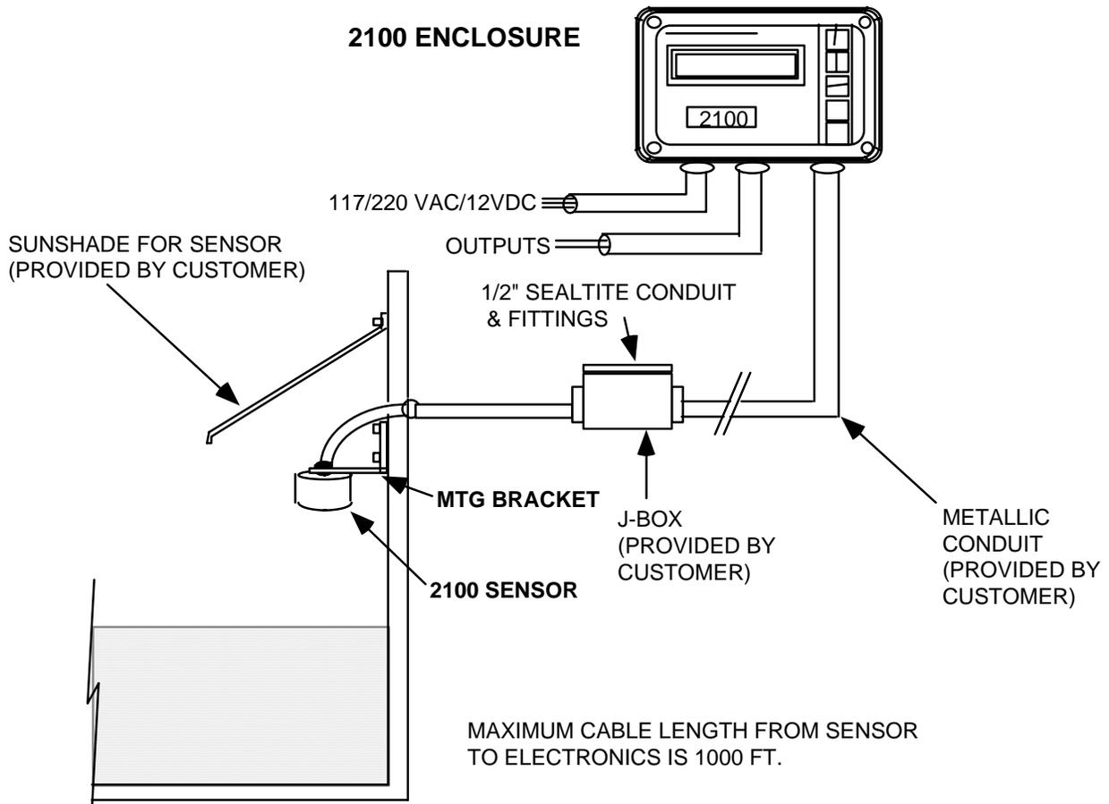
**NOTE:** 4-20 mA output must be in metallic conduit which does not contain any AC power, controller/driver, or relay wiring.
