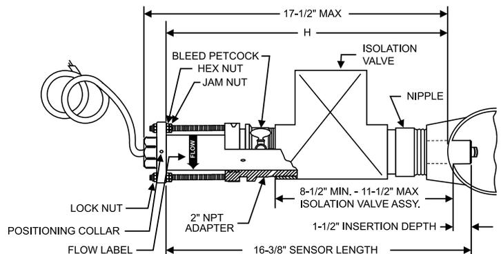
**NOTE: ALL DIMENSIONS ARE FOR REFERENCE ONLY. TO REMOVE THE FLOW SENSOR THERE MUST BE 35" OF CLEARANCE ABOVE THE OUTSIDE WALL OF THE PIPE. A CUTTING TOOL MAY REQUIRE ADDITIONAL CLEARANCE.**
