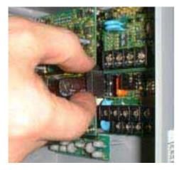
Pull out the card relay from socket
