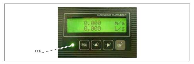
LED display: Indicates whether the received wave is normal or not.
