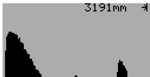
The small echo that shows in the above picture between the transmission and the proper return echo might at some stage start to confuse the instrument and cause false readings.
