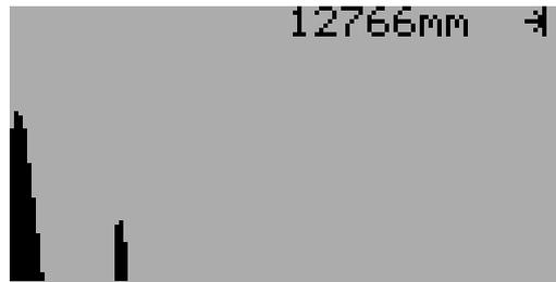
This indicates an echo pattern as seen by the instrument. From left to right, the first "column" indicates the transmit pulse and the second "column" indicates the return echo. The distance displayed in the top right corner of the display indicates the distance for the end of the screen. The user can calculate from this displayed distance where the echo signals are positioned.
