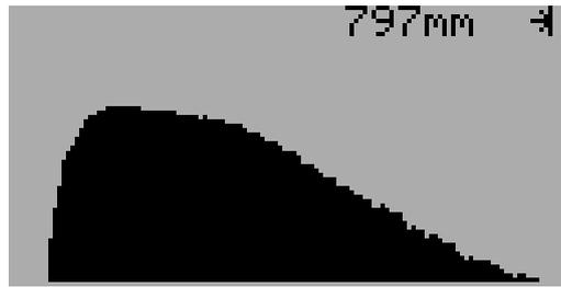
The downward slope is smooth showing that the installation was properly done. The assumption here is that the level is at least 600mm/2 ft away. Closer targets will show up in the ring-down, and the issue of whether the mounting was done properly, will be confused.
