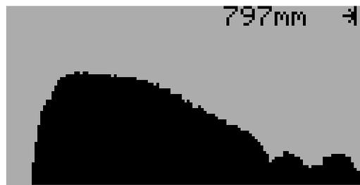
Obstructions in the path should also be checked; if no extra echoes appear between the transmit signal and the return echo, this shows that the echo path is clear from obstructions. Obstructions could be pipes, ladders, stirrers and the like. An example of a “non-clean” echo path would be as follows:
