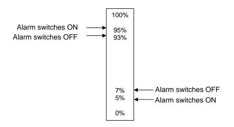
In the above, the alarm will go off at a Process Value of 95% and will only stop once the PV drops down to 93% again. On the bottom end, the alarm goes off at a Process Value of 5% and will only stop once the PV rises to 7% again.
