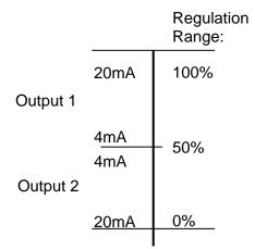
Meaning that Output 1 and Output 2 are mutually exclusive, if the PID response is in the 100% to 50% domain, then Output 1 is active and Output 2 is 4mA, if the response is in the 50% to 0% domain, then Output 1 is 4mA and Output2 is active.
