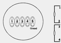
Contact rating 15VA Maximum Voltage 150VDC
