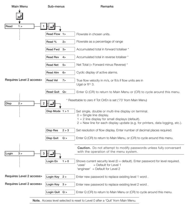
**Information.** THE FOLLOWING PARAMETERS REQUIRE 'LEVEL 1' OR 'LEVEL 2' ACCESS. (Enter passwords in 'Login En' parameter above).
