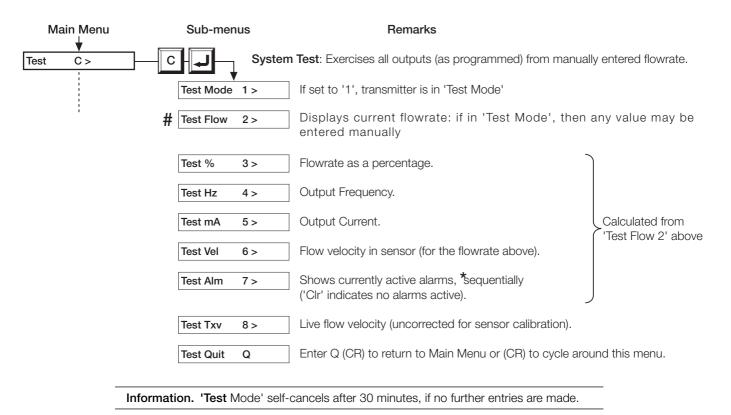
\* If the sensor is empty or disconnected, the alarms 'MtSnsr' and Coil will be displayed as appropriate.
