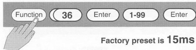
Program 1 to 99 ms. Certain electromagnetical devices require wider pulse widths. Factory default is 15 ms which should be adequate for most applications. High frequency output pulses require narrower pulse widths.
