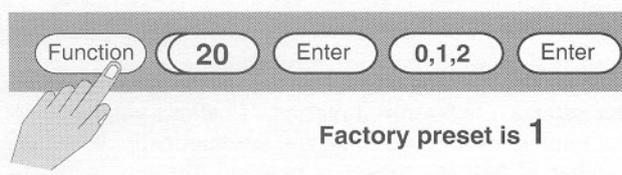
This function is programmed to view the rate of flow in units per second, minutes or hours. Code 0 is for seconds, 1 is for minutes, and 2 is for hours. To view rate of flow, simply press key number 5. To return to batch count, press key number.
