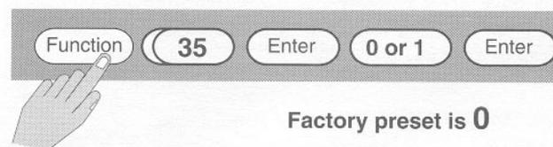
Program 0 to transmit and receive batch data or, program 1 to transmit only scaled pulses in serial form. When programmed to 1, all printer functions are disabled. Use code 1 only if the controller requires a pulse input instead of data.
