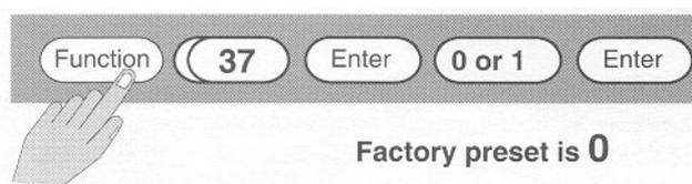
The choices are two; Code 0 will cause the output to stop if the rate returns to within setpoints. With code 1, the output will not stop until the end of the batch or until you press STOP. The rate output can be connected to an alarm to indicate overflow or underflow conditions.
