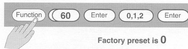
This function must be programmed to match the communications speed rate of the printer or controller.
