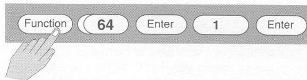
Program 1 to print at any time. This function can also be operated remotely, at any time, with a switch connection between terminals #12 and #16.
