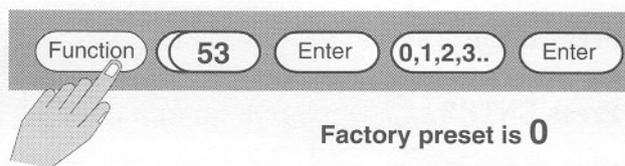
This function must be programmed if the scale factor was set up for fractions of a gallon, liter, etc. To program, simply enter the number of decimal points required on the display.
