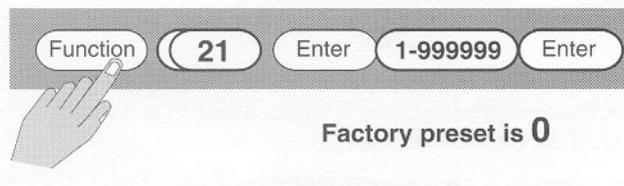
Use this function to preset a minimum flow rate. If the rate falls below the setpoint, transistor on terminal #7 will be energized. On startup, the PC100 will wait until the minimum flow is reached before activating this function.
