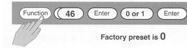
This function is used to disable the front panel START command. Program the code to 1 to disable. Once disabled, this function cannot be operated through the front panel nor remotely. Disable START only when using the PC100 as a nonresettable totalizer.
