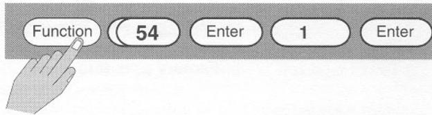
Function #54 allows you to reset the cycle counter (number of batches run) at any time. If function #15 is programmed to a preset number, the cycle counter is reset automatically when the preset number is reached. To reset, press FUNCTION-54-ENTER-1-ENTER.
