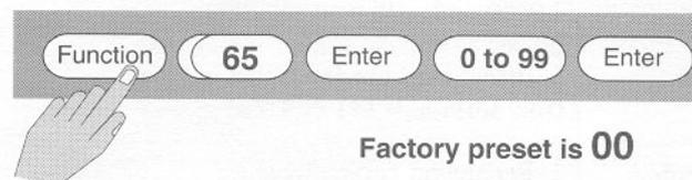
When connecting more than one PC100 to a process controller, program this function to assign an I.D. (1 to 99 to each PC100). The I.D. can then be used to channel communications from and to the host controller.
