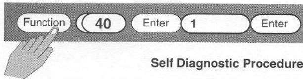
What this will do is put the PC100 into a self test of all memories and timers.
