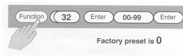
Normally, when the prewarn setpoint has been reached, the relay K1 is de-energized until the batch is terminated. However, if the prewarn signal is used to control an alarm or a feed pump, the signal duration can be programmed from 1 to 99 seconds. Never use the time out if K1 is connected to the first stage of a valve.
