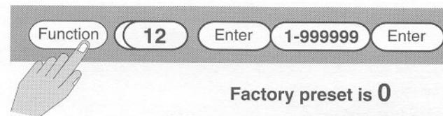
This function is used to program a limit to the size of batch that can be entered. This will prevent over batching. Example: If the largest allowable batch in your operation is 255 gallons, then program the batch limit to 255 gallons.
