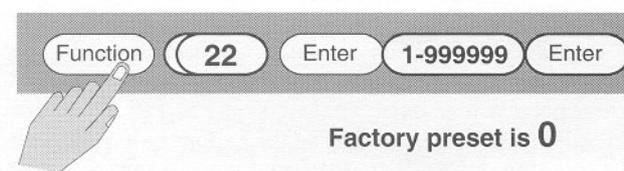
Use this function to preset a maximum flow rate. If the rate exceeds the setpoint, transistor on terminal #7 will be energized. Use the output to activate an alarm or other indication devices.
