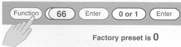
Printers often require different delay periods between lines of information transmitted. This function must be programmed to match the required line print delay of your printer. Program 0 for 0.1 second and 1 for 1 second.
