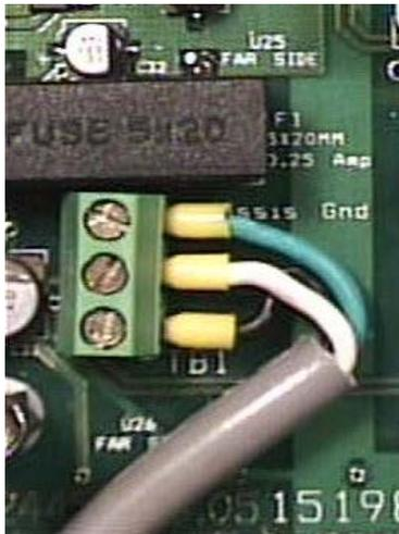
AC power is clearly marked in the terminal block labelled TB1 located under the front panel. The unit is designed to handle voltage from 90 to 240 VAC. The unit requires 5 VA for proper operation. Proper personnel shall wire the unit in accordance with local codes.
