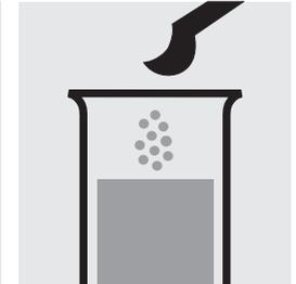
Add 1 level blue microspoon of **NH<sub>4</sub>-2** (from Spectroquant® Ammonium Test, Cat. No. 114752).
