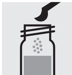
Add 1 level yellow micro-spoon of **NO<sub>3</sub>-1K** into a reaction cell and close with the screw cap.
