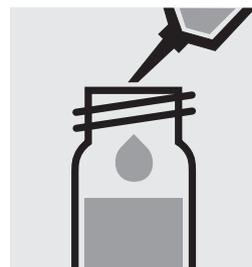
Add 1.0 ml of **N-3K** with pipette, close the cell with the screw cap, and mix. **Caution, cell becomes hot!**
