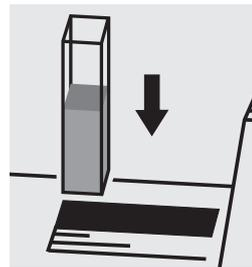
Place the cell into the cell compartment.
