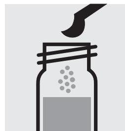
Add 1 level green microspoon of **CN-3**, close the cell with the screw cap.
