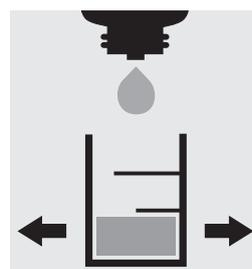
Check the chloride content of the depleted sample using MColorTest™ Chloride Test (Cat. No. 111132) according to the application (see the website): specified value <250 mg/l Cl<sup>-</sup>.
