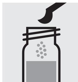
Add 1 level blue micro-spoon of **F-1K**, close the cell with the screw cap.
