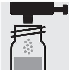
At the first use replace the black screw cap of the reagent bottle by the dose-metering cap.
