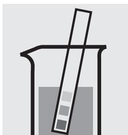
Check the pH of the sample, specified range: pH 3 – 8. If required, add dilute sodium hydroxide solution or sulfuric acid drop by drop to adjust the pH.
