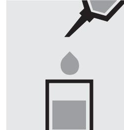
Transfer the solution into the quartz cell.
