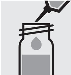
**Carefully** pipette 2.0 ml of the sample into a reaction cell, close tightly with the screw cap, and mix vigorously. **Caution, the cell becomes hot!**
