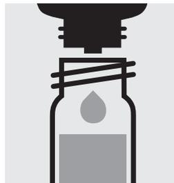
Add 3 drops of **H-2K** to the already measured cell, close the cell with the screw cap, and mix.
