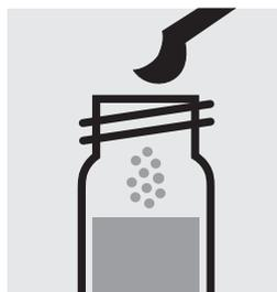
Add 1 level blue microspoon of **CN-1K**, close the cell with the screw cap.
