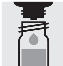
Add 5 drops of **P-1K**, close the cell with the screw cap, and mix.
