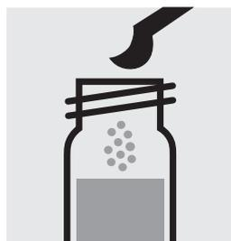
Add 1 level yellow micro-spoon of **N-3K** into a **reaction cell**, close the cell with the screw cap.
