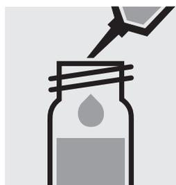
Pipette 6.0 ml of the sample into a reaction cell, close with the screw cap, and mix.
