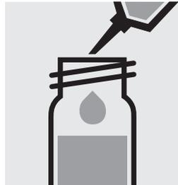
Carefully pipette 5.0 ml of the **depleted sample** into a reaction cell, close tightly with the screw cap, and mix vigorously. **Caution, the cell becomes hot!**
