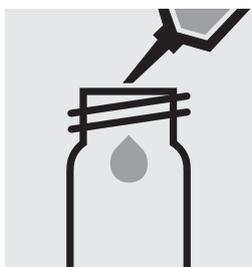
Pipette 10 ml of the sample into a round cell (Empty cells, Cat.No. 114724).
