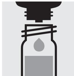
Add 3 drops of **CN-2K**, close with the screw cap, and mix: **pretreated sample**.
