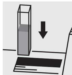
Place the cell into the cell compartment.
