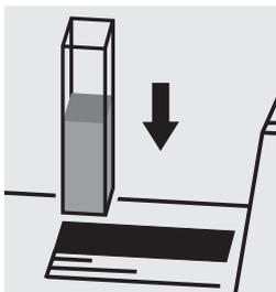
Place the cell into the cell compartment. Select method no. 305.
