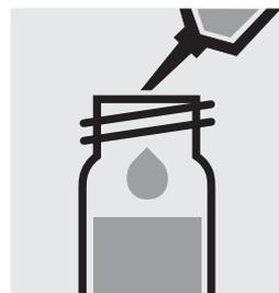
Add 5.0 ml **Isobutyl-methylketone GR** (Cat.No. 106146) with pipette, close the cell with the screw cap.
