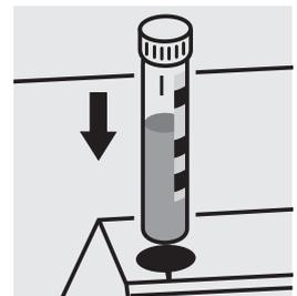
Place the cell into the cell compartment. Align the mark on the cell with that on the photometer.
