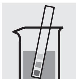
Check the pH of the sample, specified range: pH 0–10. If required, add dilute sulfuric acid drop by drop to adjust the pH.
