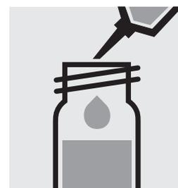
Add 3.0 ml of the sample with pipette, close the cell with the screw cap, and mix. **Caution, cell becomes hot!**
