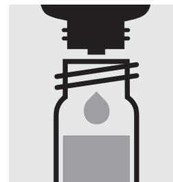
Add 2 drops of **Ni-2K**, close the cell with the screw cap, and mix.
