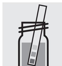
Check the pH of the sample, specified value: pH 3.0. If required, add dilute sodium hydroxide solution or sulfuric acid drop by drop to adjust the pH.
