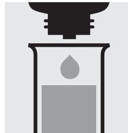
Add 4 drops of **NH<sub>4</sub>-3** (from Spectroquant® Ammonium Test, Cat. No. 114752) and mix.
