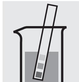
Check the pH of the sample, specified range: pH 3–6.
