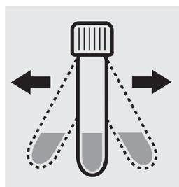
Shake the cell vigorously for 1 minute. Leave to stand to allow phases to separate.
