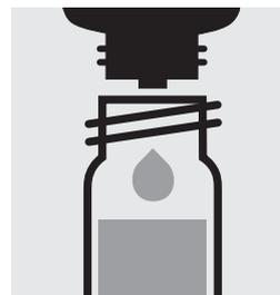
Add 2 drops of **Ni-1K**, close with the screw cap, and mix.
