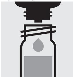
Add 5 drops of **Zn-3**, close the test tube with the screw cap, and mix.
