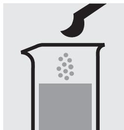
Add 1 level green micro-spoon of **Zn-1K** and shake to dissolve the solid substance: **sample-reagent mixture**.
