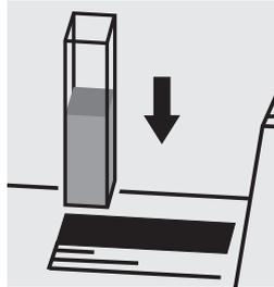
Place the cell into the cell compartment.
