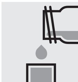
Transfer the solution into a rectangular cell.
