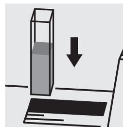
Place the cell into the cell compartment.
