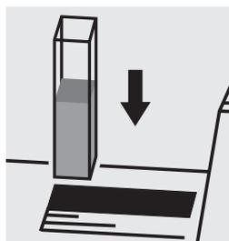
Place the cell into the cell compartment.
