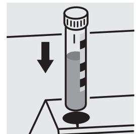
Place the cell containing the sample into the cell compartment. Align the mark on the cell with that on the photometer.
