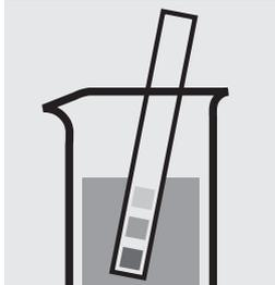
Check the pH of the sample, specified range: pH 3 – 11. If required, add dilute sodium hydroxide solution or sulfuric acid drop by drop to adjust the pH.
