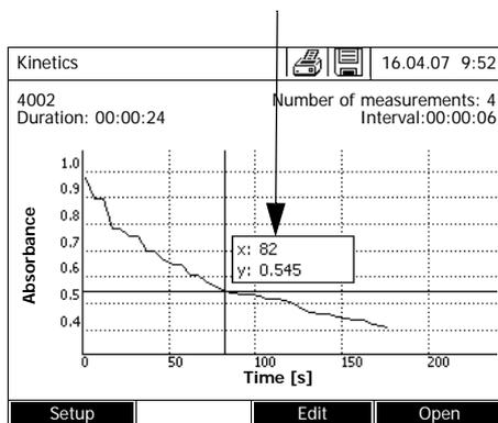
The cursor consists of a horizontal and vertical line that cross each other on a point of the curve. A box names the x and y values of the point of the curve.
