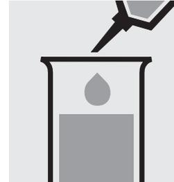
Add 0.60 ml of **NH<sub>4</sub>-1** (from Spectroquant® Ammonium Test, Cat. No. 114752) with pipette and mix.
