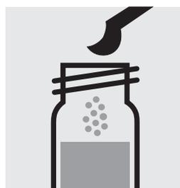
Add 1 level blue micro-spoon of NO<sub>3</sub><sup>-</sup>-1, **immediately** close tightly with the screw cap.
