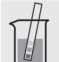
Check the pH of the sample, specified range: pH 2 – 7. If required, add dilute sodium hydroxide solution or sulfuric acid drop by drop to adjust the pH.
