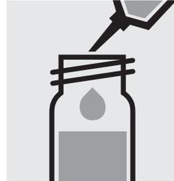
Add 0.20 ml of **Cd-1K** with pipette, close the cell with the screw cap, and mix.
