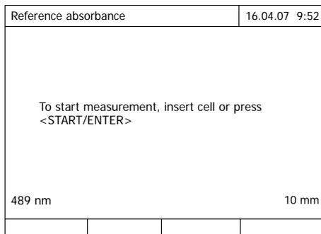
**2** Insert the cell with the reference sample.
