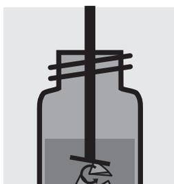
Disintegrate the filter in the homogenizer.
