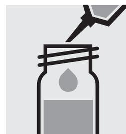
Add 0.20 ml of **reagent 2** with pipette, close the cell with the screw cap, and mix.
