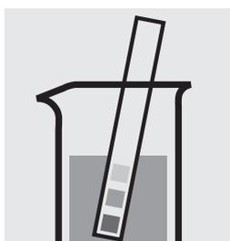
Check the pH of the sample, specified range: pH 1 – 12. If required, add dilute ammonia solution or nitric acid drop by drop to adjust the pH.
