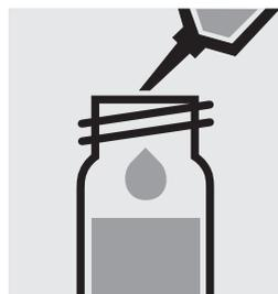
Pipette 1.0 ml of the **pretreated sample** into a reaction cell, **do not mix!**
