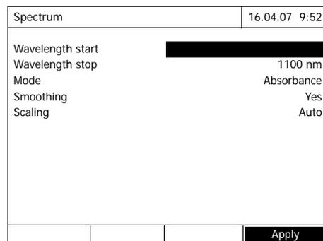
2 Select the start and end point of the spectrum to be recorded and the mode (*Absorbance* or *Transmission*).
