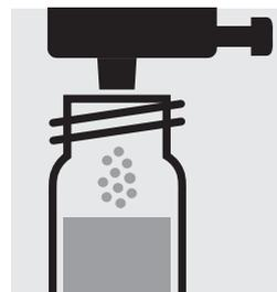
Add 1 dose of **Cr-2K** using the blue dosing cap, close the reaction cell with the screw cap.
