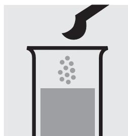
Add 1 level blue microspoon of **Al-1** to the test tube and dissolve the solid substance.
