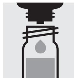
Add 6 drops of **N-2K**, close the cell with the screw cap, and mix.
