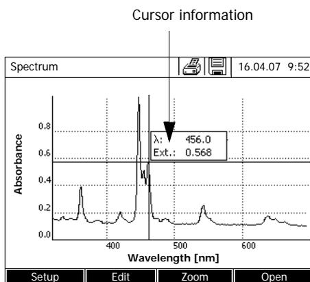
The cursor consists of a horizontal and vertical line that cross each other on a point of the curve. A box names the x and y values of the point of the curve.
