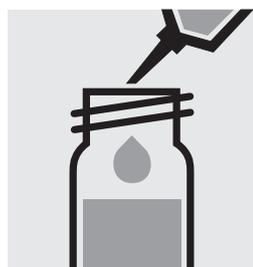
Pipette 2.0 ml of the sample into a reaction cell, close with the screw cap, and mix.
