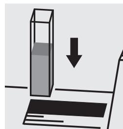
Place the cell into the cell compartment.
