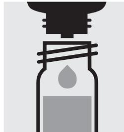
Add 5 drops of **Pb-1K** into a reaction cell and mix.
