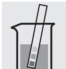
Check the pH of the sample, specified range: pH 3 – 9.
