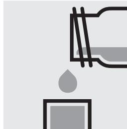
Transfer the solution (when possible without sediment) into a corresponding rectangular cell.
