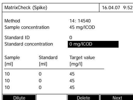
If the spiking with the standard values of the CombiCheck R-2 suggested by the photometer would cause the measuring range to be exceeded, the MatrixCheck by diluting is automatically suggested.
