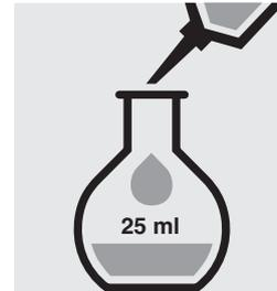
Add 1.0 ml of **reagent 3** with pipette, fill to the mark with distilled water, and mix thoroughly.
