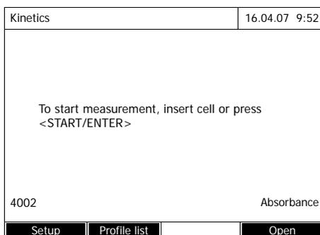
The photometer is ready to measure after the profile has been selected.
