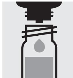
Add 3 drops of **Zn-4**, close the test tube with the screw cap, and mix.
