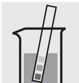
Check the pH of the sample, specified range: pH 4 – 13. If required, add dilute sodium hydroxide solution or sulfuric acid drop by drop to adjust the pH.
