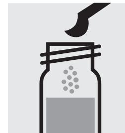
Add 1 level grey micro-spoon of **Zn-5**, close the test tube with the screw cap, and dissolve the solid substance.
