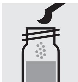
Add 1 level blue microspoon of **CN-4**, close the cell with the screw cap.
