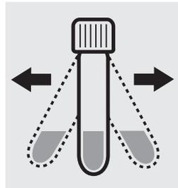
Shake the cell **vigorously for 5 seconds** to dissolve the solid substance.
