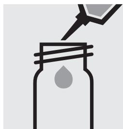
Pipette 10 ml of the sample into an empty round cell (Empty cells, Cat.No. 114724).
