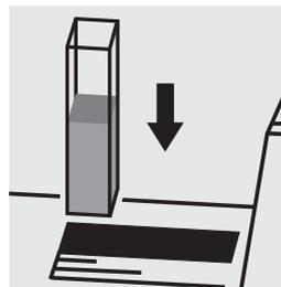
Place the cell into the cell compartment.
