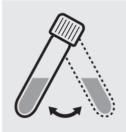
Suspend the bottom sediment in the cell by swirling.
