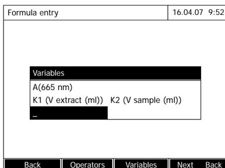
**11** Select and confirm the Variable  $A_{665\text{ nm}}$  for the second measurement.
