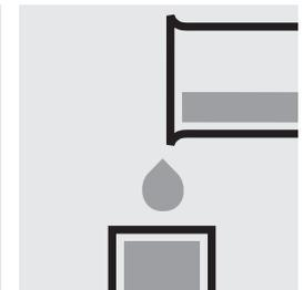
Transfer the solution into a corresponding cell.
