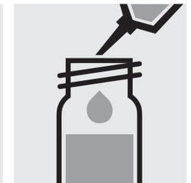
Add 5.0 ml of **Zn-6** (Cat.No. 106146, Isobutyl-methylketone) with pipette and close the test tube with the screw cap.
