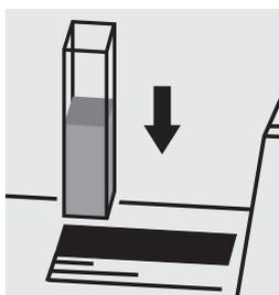
Place the cell into the cell compartment.
