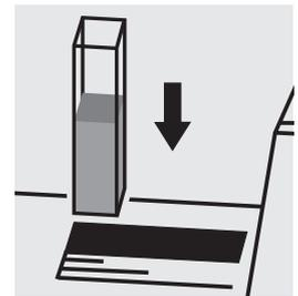
Place the cell into the cell compartment.
