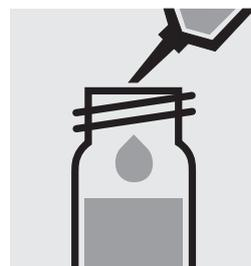
Add 3.0 ml of the sample with pipette, close the cell with the screw cap, and mix.
