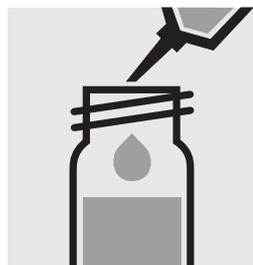
Add 0.25 ml of **Cl-1K** with pipette, close with the screw cap, and mix.
