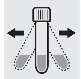
Shake the cell vigorously to dissolve the solid substance.
