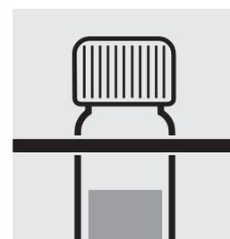
Remove the cell from the thermoreactor and place in a test-tube rack to cool to room temperature: **pretreated sample**.
