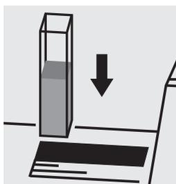
Place the cell into the cell compartment.
