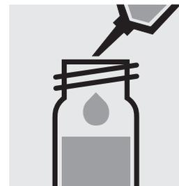
Add 7.0 ml of the sample with pipette to one reaction cell, close with the screw cap, and mix.
