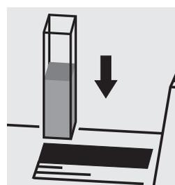
Place the cell into the cell compartment. Select method no. **2517** or **2518**.
