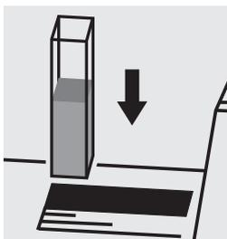
Place the cell into the cell compartment.
