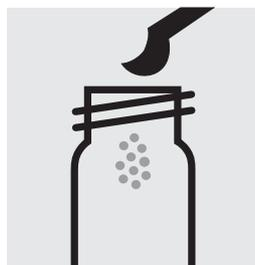
Place 1 blue micro-spoon of **NO<sub>3</sub>-1** into a dry empty round cell (Empty cells, Cat.No. 114724).
