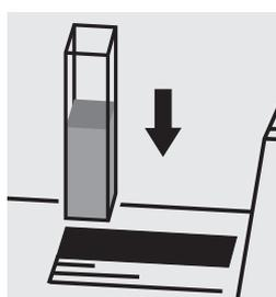
Place the cell into the cell compartment, select method no. **15**, **61**, or **78**.
