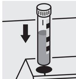
Place the cell into the cell compartment. Align the mark on the cell with that on the photometer = **Result B**
