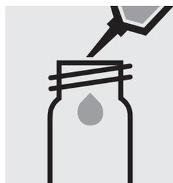
Pipette 10 ml of distilled water (Water Ultrapur, Cat.No. 101262, is recommended) into a second plastic vessel (**Flat-bottomed tubes, Cat.No. 117988**). (Blank)
