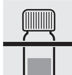
Remove the cell from the thermoreactor and place in a test-tube rack to cool.
