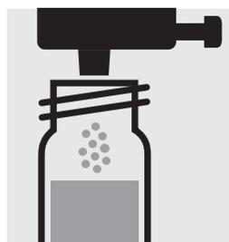
Add 1 dose of **CN-1** using the green dosing cap, close the cell with the screw cap.
