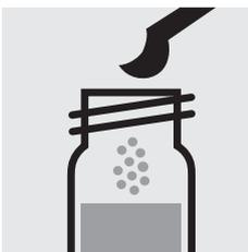
Solid substances are dosed either with the dose-metering cap or with microspoons that are integrated into the screw cap of the respective reagent bottle. The dose-metering cap is used for solid reagents or reagent mixtures that are free-flowing.
