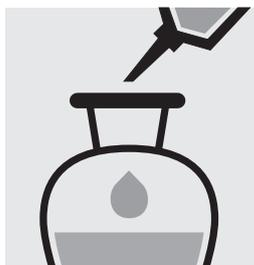
Pipette 200 ml of sample into a separation funnel.
