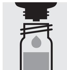
Add to each vessel 3 drops of **Si-1**, close with the screw cap, and mix.
