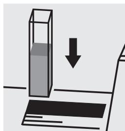
Place the cell into the cell compartment.
