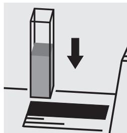
Place the cell into the cell compartment.
