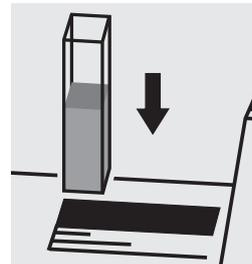
Place the cell into the cell compartment.
