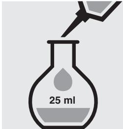
Pipette 4.0 ml of the sample into a 25-ml volumetric flask, fill to the mark with distilled water and mix thoroughly.
