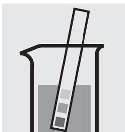
Check the pH of the sample, specified range: pH 2 – 8.
