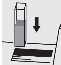
Place the cell into the cell compartment, select method no. **21**.
