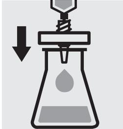
Filter sample solution through a membrane filter with 0.45 µm pore size.
