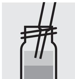
Aspirate the organic-clear upper phase from the tube with pipette and dry over **sodium sulfate anhydrous** (Cat.No. 106649).
