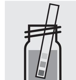
Check the pH, specified range: pH 12–13. If required, add dilute sodium hydroxide solution drop by drop to adjust the pH.
