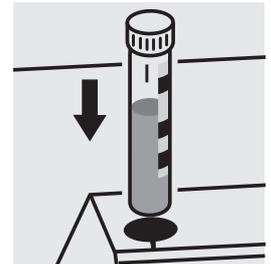
Place the cell into the cell compartment. Align the mark on the cell with that on the photometer = **Result total hardness**
