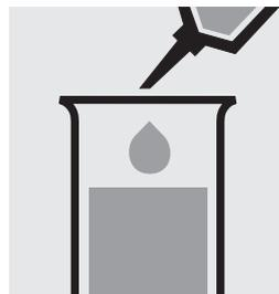
Pipette 5.0 ml of distilled water (Water for analysis EMSURE<sup>®</sup>, Cat.No. 116754, is recommended) into a test tube.
