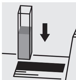
Place the cell into the cell compartment.
