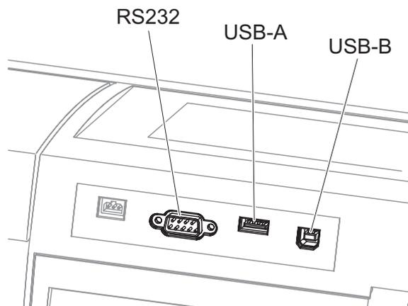
figure 3-1 Communication interfaces on the rear panel
