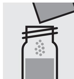
Add 1 powder pack of **Molybdenum HR3** and close with the screw cap.
