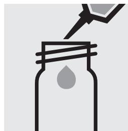
Pipette 5.0 ml of the sample into an empty round cell (Empty cells, Cat.No. 114724).
