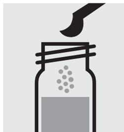
Add 1 level grey micro-spoon each of  **$\text{SO}_3$ -1K** into two reaction cells, close with the screw cap.
