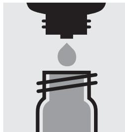
Add 10 drops of O<sub>2</sub>-3K, close the cell with the screw cap, mix, and clean from outside.
