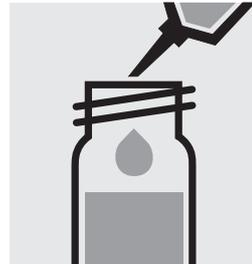
Carefully pipette 3.0 ml of the **depleted blank** into a second reaction cell, close tightly with the screw cap, and mix vigorously. **Caution, the cell becomes hot!**
