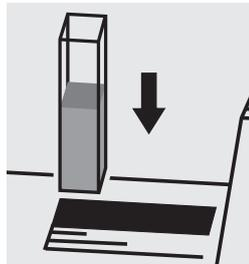
Place the cell into the cell compartment.
