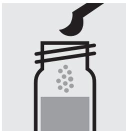
Add 1 level grey micro-spoon of **Pb-2K** to the already measured cell, close the cell with the screw cap.
