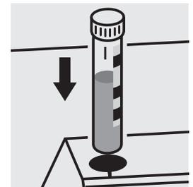
Place the cell into the cell compartment. Align the mark on the cell with that on the photometer = **Result A**
