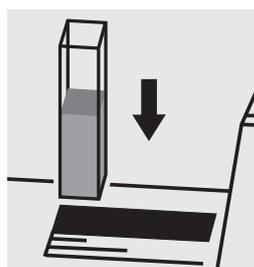
Place the cell into the cell compartment.
