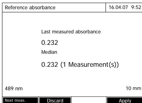
**3** If necessary, carry out further single measurements for the formation of the median with *[Next meas.]* or discard the last single measurement with *[Discard]*.
