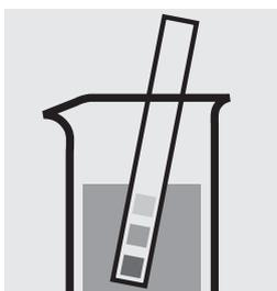
Check the pH of the sample, specified range: pH 4 – 10.
