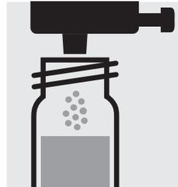
Add 1 dose of **F-1K** using the blue dose-metering cap, close the cell with the screw cap.
