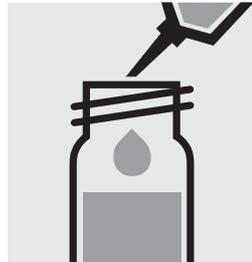
Carefully pipette 5.0 ml of the **depleted blank** into a second reaction cell, close tightly with the screw cap, and mix vigorously. **Caution, the cell becomes hot!**
