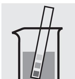
Check the pH of the sample, specified value: pH 7.0. If required, add dilute sodium hydroxide solution or sulfuric acid drop by drop to adjust the pH.
