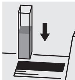
Place the cell into the cell compartment.
