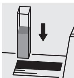
Place the cell into the cell compartment.
