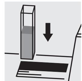
Place the cell into the cell compartment.
