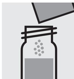
Add 1 powder pack of **Molybdenum HR2**, close with the screw cap, and dissolve the solid substance.
