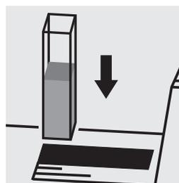
Place the cell into the cell compartment.
