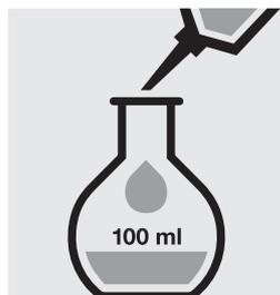
Pipette 4.0 ml of the dilute sample into a 100-ml volumetric flask, fill to the mark with distilled water and mix thoroughly.
