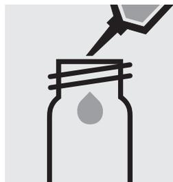
Pipette 5.0 ml of the 1:4 dilute sample into an empty round cell (Empty cells, Cat.No. 114724).
