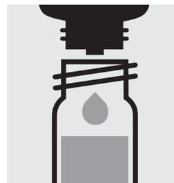
Add 5 drops of **Zn-2K**, close the cell with the screw cap, and mix.
