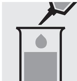
Add 1.0 ml of **reagent 1** with pipette and mix.
