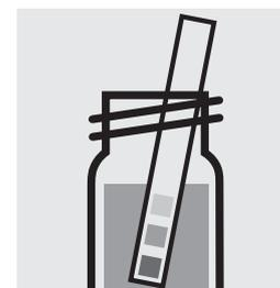
Check the pH of the sample, specified value: pH 6.5. If required, add dilute sodium hydroxide solution or sulfuric acid drop by drop to adjust the pH.
