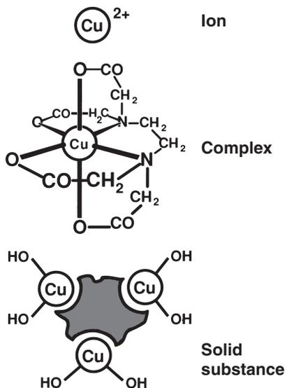
Water-borne substances can be present in the sample for investigation in a variety of forms: as the ion, bound more or less solidly in a complex, or as a solid substance.
