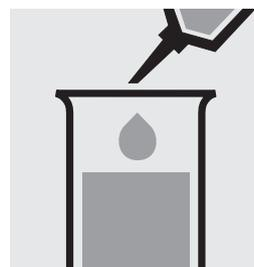
Add 0.50 ml of **PO<sub>4</sub>-1** with pipette and mix.
