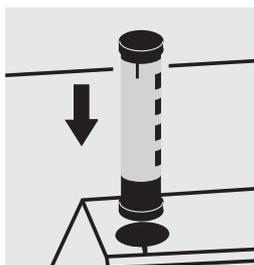
Select method with AutoSelector measuring range 10 – 250 mg/l Cl.
