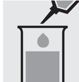
Pipette 5.0 ml of distilled water (Water for analysis EMSURE<sup>®</sup>, Cat.No. 116754, is recommended) into a second test tube. (Blank)
