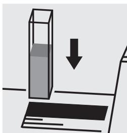
Place the cell into the cell compartment. Select method no. 20.
