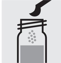
Add 1 level green micro-**spoon** of **HCHO-1K** into a reaction cell, close with the screw cap.
