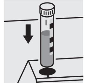
Place the cell into the cell compartment. Align the mark on the cell with that on the photometer.
