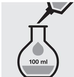
Pipette 5.0 ml of the sample into a 100-ml volumetric flask, fill to the mark with distilled water and mix thoroughly.
