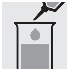
Pipette 0.10 ml of the sample into a test tube.
