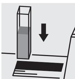
Place the cell into the cell compartment.
