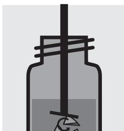
Disintegrate the filter in the homogenizer. Rinse together with a small portion of ethanol.
