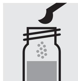
Add 1 level green microspoon of **Ag-2**, close the cell with the screw cap.
