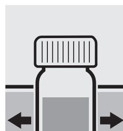
Temper the test tube again in the water bath for 7 minutes.
