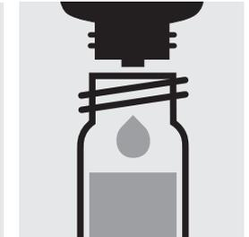
Add 2 drops of **Zn-2**, close the test tube with the screw cap, and mix.
