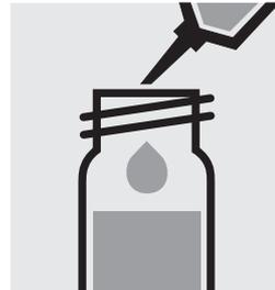
**Immediately** add 1.5 ml of **NO<sub>3</sub>-2** with pipette.
