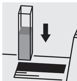
Place the cell into the cell compartment.
