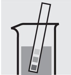
Check the pH of the sample, specified range: pH 1 – 10. If required, add dilute sodium hydroxide solution or sulfuric acid drop by drop to adjust the pH.
