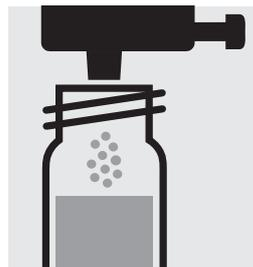
Add 1 dose of **P-3K** using the blue dosing cap, close the cell with the screw cap.
