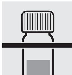
Replace both cells in the rack for complete cooling to room temperature. **(Very important!)**
