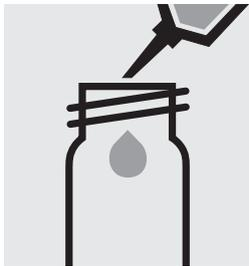
Pipette 10 ml of the sample into into a empty round cell (Empty cells, Cat.No. 114724).
