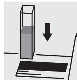
Place the cell into the cell compartment.
