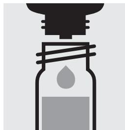
Add 6 drops of **Sn-1K** into a reaction cell, close with the screw cap, and mix.
