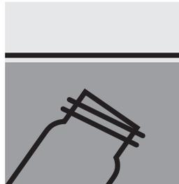
Fill watersample into a reaction cell to overflowing and make sure, that no air bubbles are present.
