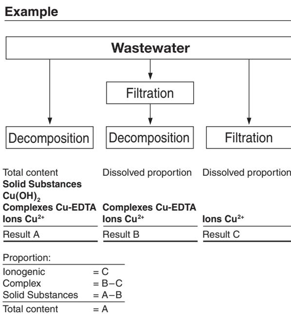
Decomposition converts the substance to be determined into an analyzable form. In most cases, decomposition agents take the form of acids in combination with oxidizing agents; in exceptional cases (e. g. in the determination of total nitrogen) an alkaline decomposition is more effective. The type of decomposition procedure used depends on the analyte to be determined and the sample matrix.
