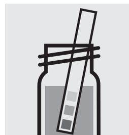
Check the pH, specified range: pH 4–10. If required, add dilute sodium hydroxide solution or sulfuric acid drop by drop to adjust the pH.
