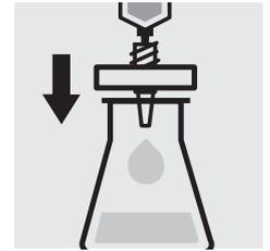
Filter the contents of the syringe into the intended glass vessel.
