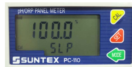
After Cal. slope status for the diagnosis index of the sensor
