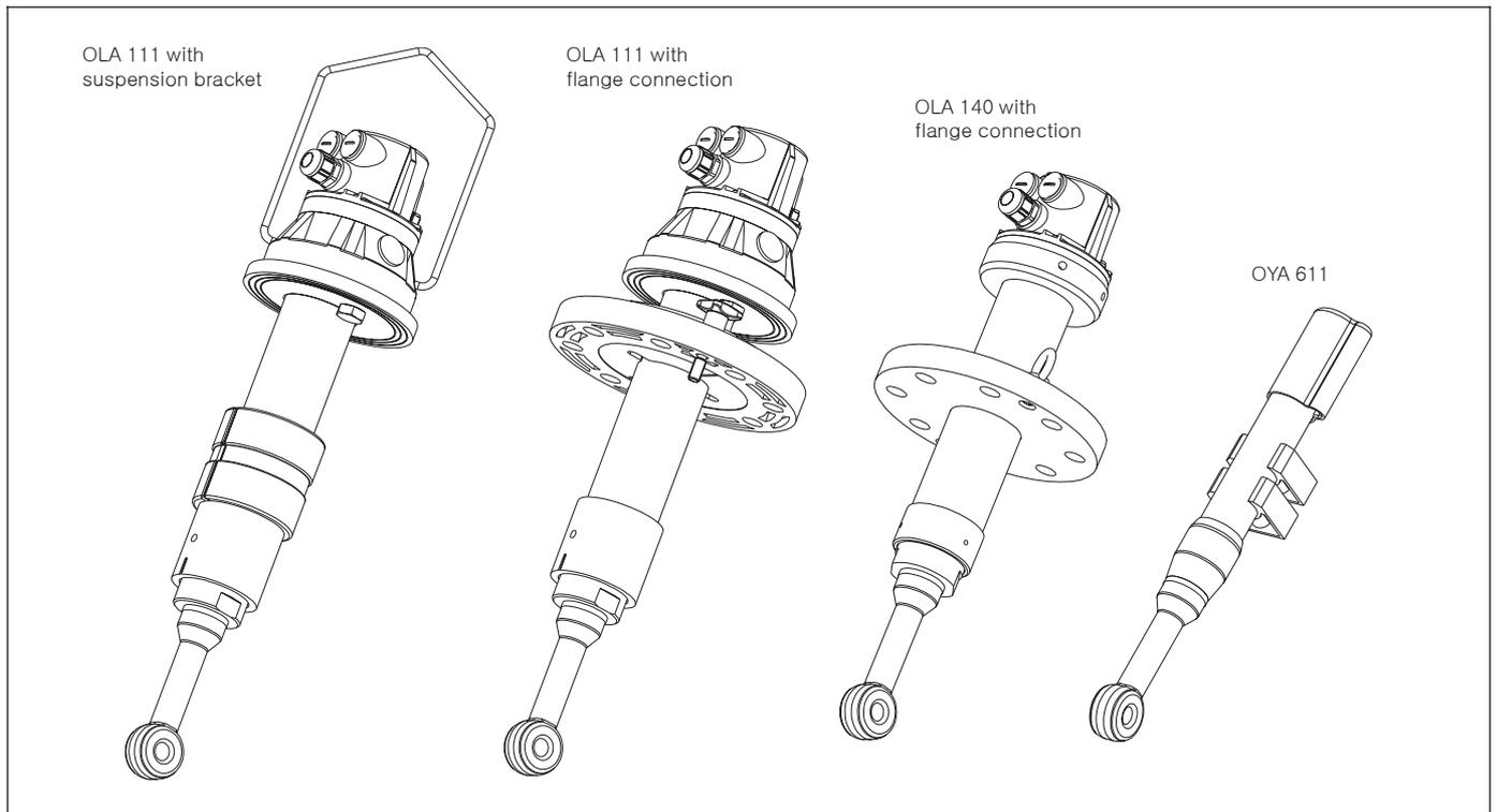
Assembly mounting of measuring cell, G 3/4 version
