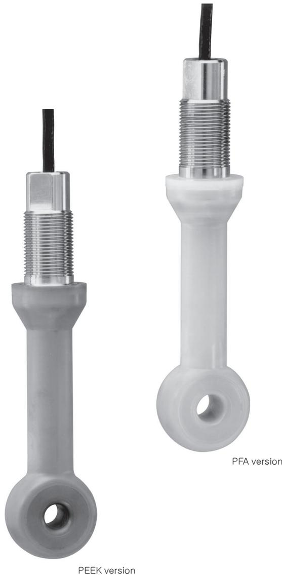
The conductivity sensor OLS 50 is specially suitable for use in the chemical industry and in process engineering. The six-decade measuring range and high chemical resistance of the material in contact with the medium (PFA or PEEK) permit this sensor to be used in virtually any application conceivable. The wide temperature range of  $-20$  to  $+125$  °C ( $+180$  °C) leaves nothing to be desired.
