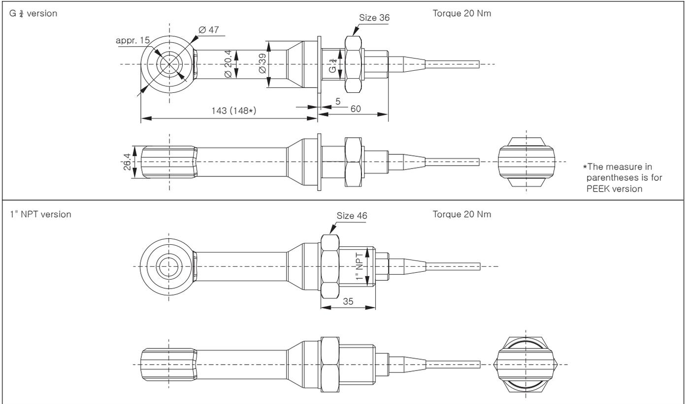
Dimensions: Versions with G 3/4 thread (top) and 1" NPT thread (bottom)
