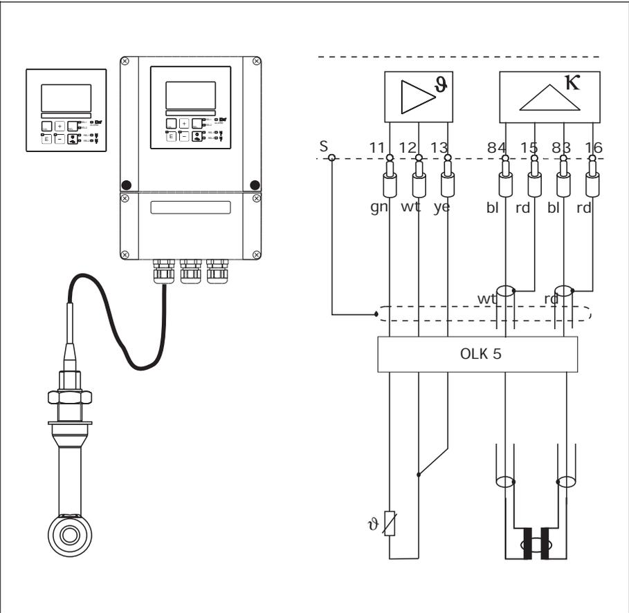
Cable connection at transmitter OLM 223/253
