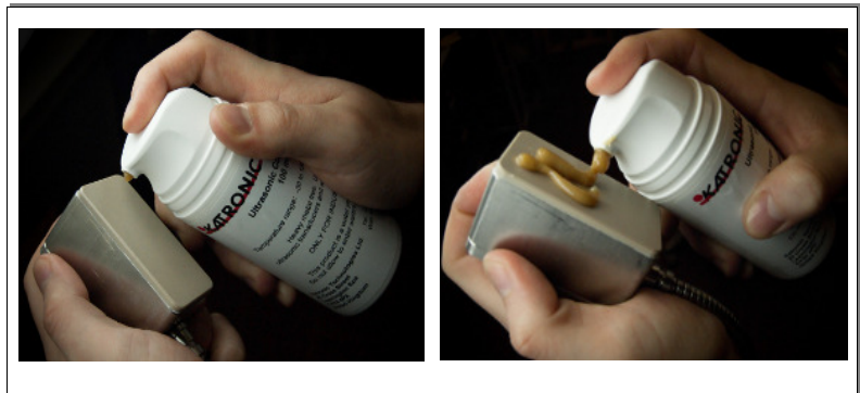
Illustration 5: Application of acoustic coupling gel
