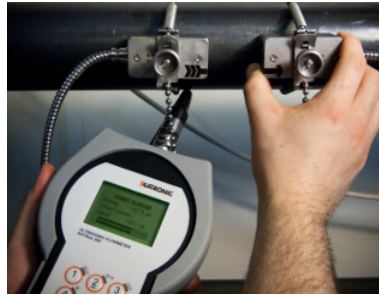
Illustration 6: Correct positioning of the sensors
