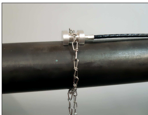
PT100 sensor fixed to pipe
