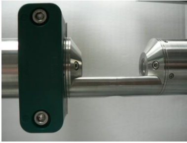
Mechanical sensor-holding system (front view)
