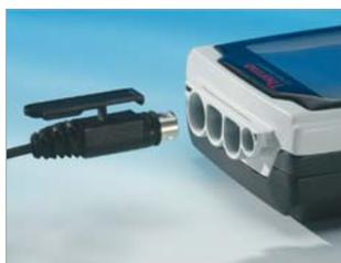
If you have ever lost data – or even an electrode – because of a failed connection, you'll appreciate the Orion Star Series' proprietary waterproof BNC and MiniDIN locking connectors. Adapter cables can be used to connect Orion Star Series electrodes to a wide variety of other meters.
