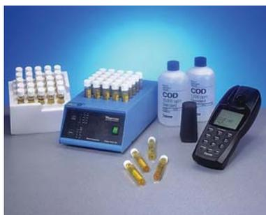
COD Reactor, Test Reagents and Standards with AQ4000 Meter
