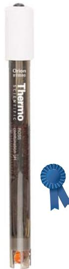
**ROSS® combination pH electrode with epoxy body**
