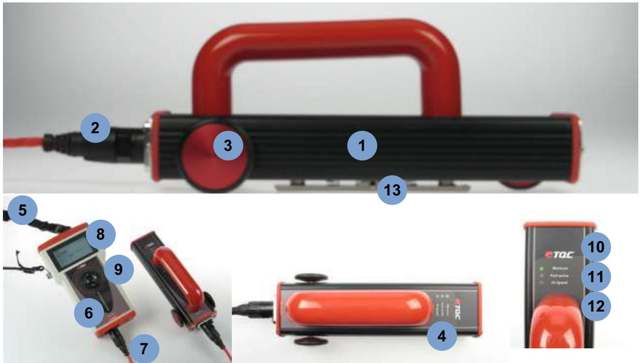
1. Hull Roughness sensor
