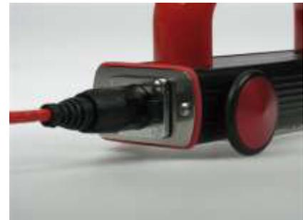
Note: To release the sensor cable from both sensor and control unit push the little fuse button beside both connectors. The plug should be able to eject from the connector without the use of excessive force.
