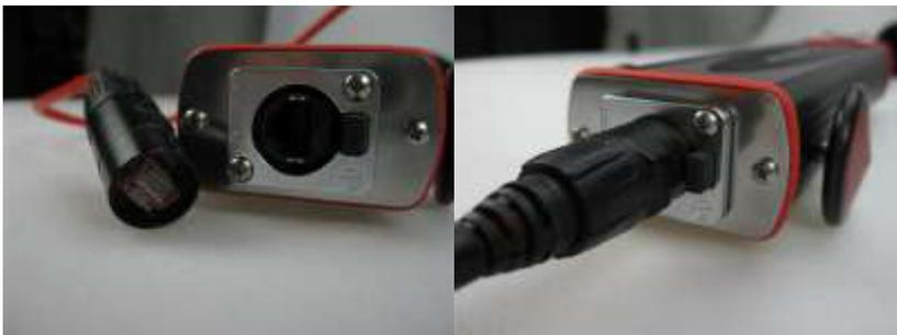
Note: To release the sensor cable from both sensor and control unit push the little fuse button beside both connectors. The plug should be able to eject from the connector without the use of excessive force.
