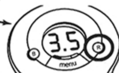
\*NOTE: Standard Method (4500-Cl G, simplified procedure for total chlorine) requires the reading to be made after a 2 minute wait. From experience, water samples above 68°F, generally, do not require the full 2 minute wait.
