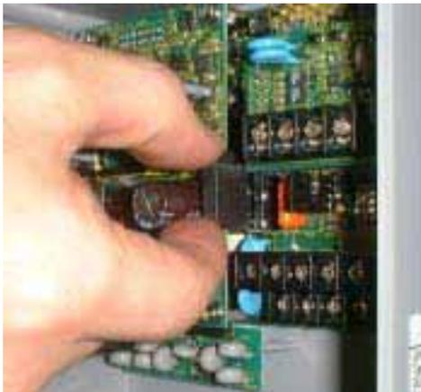
Pull out the card relay from socket
